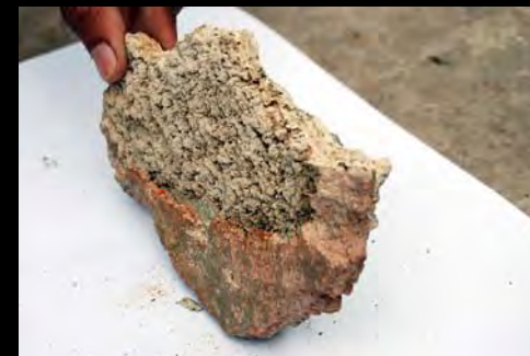
2-3 cm thick epoxy layers February 2009
