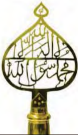
The top inscription, made in brass, was laser cut from a single brass sheet
