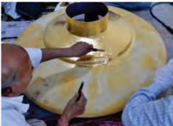
The top inscription, made in brass, was laser cut from a single brass sheet
