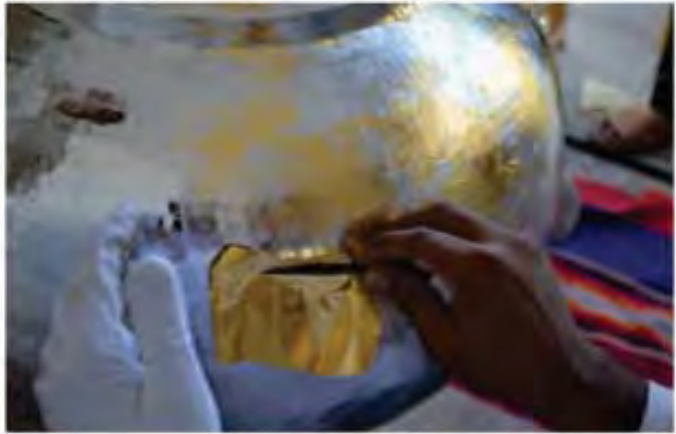
Traditional gilding process required mercury to be first applied to the clean copper vessels
